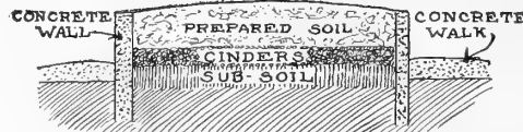
Method of providing thorough drainage for solid greenhouse bed built on the ground
